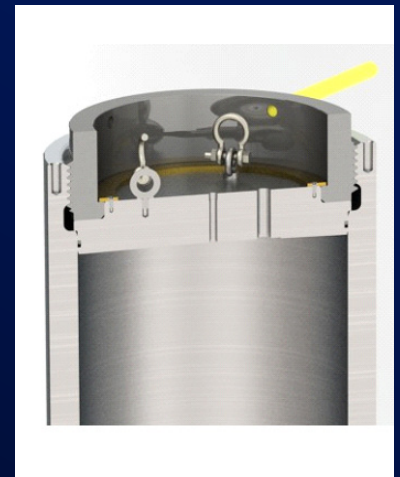
Above - Examples of simple continuous thread closure.
